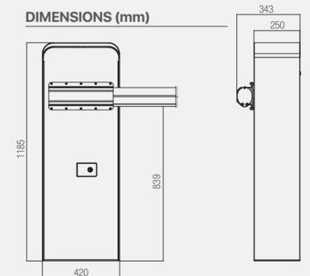
For beams up to 7 m (3+4 m) and up to 8 m (4+4 m)
